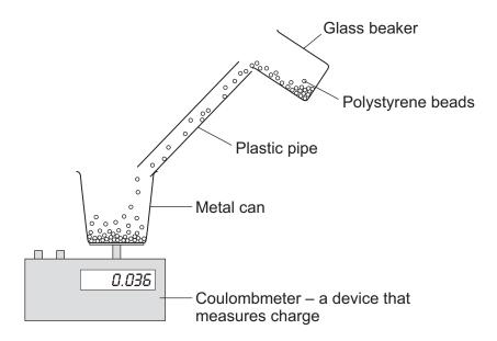
The student poured 75cm<sup>3</sup> of polystyrene beads down the pipe. The beads fell into a metal can and the charge on them was measured directly using a coulombmeter.
